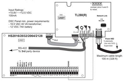
4. Install the RS-422 connections (R models only). If using the communicator with a 3rd party device, wire the connections as per the table below:
