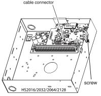
a. Disconnect both AC power and battery connections from the panel, and disconnect telephone line.
